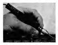
input. The LCA-2 is supplied with a 4-foot coaxial cable, BNC connector, and three input adapters. It can indicate polarity/duty cycle of pulse trains as high as 25 MHz. The probe measures 5½-in. long and ¾-in. in diameter. \$69.50.
