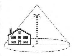
Fig. 3. A metal antenna tower, properly grounded, provides a cone of protection for the house.
