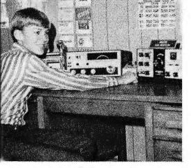
Rick, WB9EWQ, uses a Heathkit Electronic Keyer with HW-16 and HW-101 transceivers.
