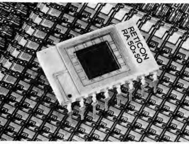
Fig. 4. Close-up of the Reticon RA 50×50 sensor. The background is photo of the array magnified many times.
