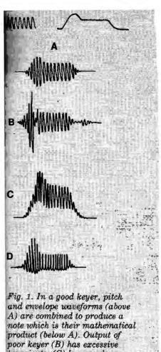
transients; (C) has envelope in output; (D) has unequal positive and negative swings.
