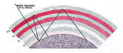
Signals may be reflected by a layer of the ionosphere or escape into space. Range is determined by layer height and wave angle.
