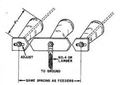
Fig. 1. A spark gap arrestor to protect ham antenna is easily made.
