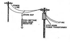
Fig. 2. In power-line arrestor, current is reduced by resistor.
