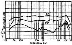
Fig. 3. Cardioid frequency response on axis and at two angles off-axis.
