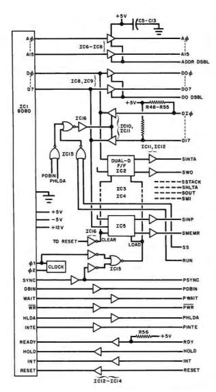
Fig. 8. The logic associated with the CPU (ICI) is shown at left. All of the buffers and latches are on a single pc board. Connecting wiring is through a 100-line buss.
