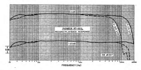
corder to be very accurate at both speeds. It was within  $\pm 0.5$  dB from 50 Hz to 15,000 Hz at 7½ ips and within  $\pm 0.8$  dB from 50 Hz to 7500 Hz at 3 ¾ ips. (These are the frequency limits of the test tapes.)
