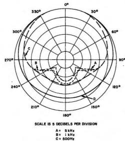
Fig. 2. Cardioid pickup patterns at four different frequencies.
