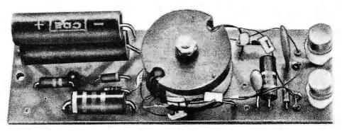
Fig. 3. Wired pc board assembly shows T1 mounted with hardware fiber washer. C4 is on top of C3.
